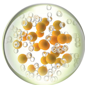
Silica monomers and drug substances are emulsified together
